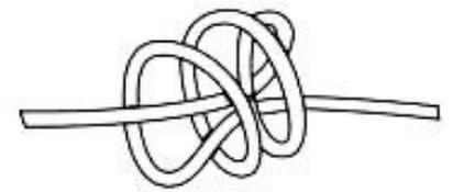
**heaving line knot**
